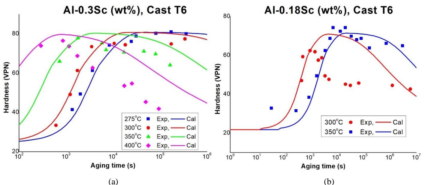
Fig. 4 Evolution of hardness with different ageing temperatures for Al-0.3Sc (wt%) [3] and Al-0.18Sc (wt%) [18] alloys at cast T6 conditions. The initial homogenization temperature was  $648^\circ\text{C}$  for Al-0.3Sc and  $640^\circ\text{C}$  for Al-0.18Sc.
