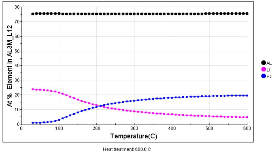
Fig. 2 Phase composition of  $Al_3M_L1_2$  of a ternary Al-Li-Sc alloy
