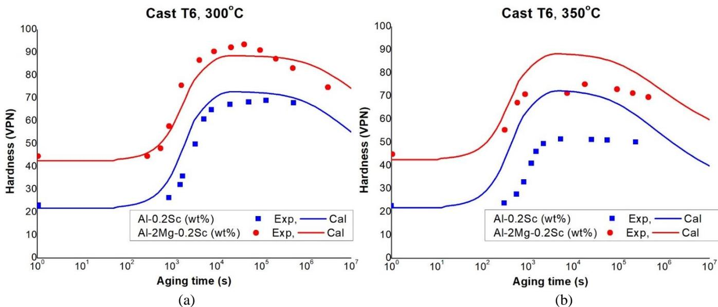
Fig. 5 Age hardening curves of binary Al-0.2Sc (wt%) and ternary Al-2Mg-0.2Sc (wt%) alloys at cast T6 condition [19]. The alloys were homogenized at 617°C, quenched into room temperature and subsequently aged at 300°C and 350°C.
