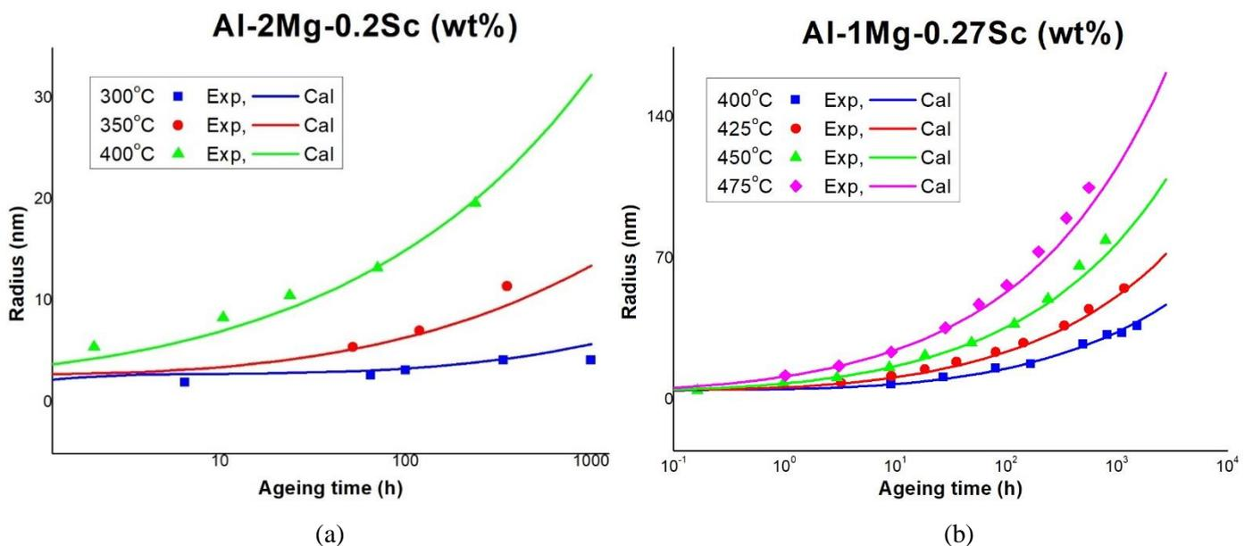
Fig. 3 Comparison between calculated and measured evolution of  $Al_3Sc$  particle radius of (a) Al-2Mg-0.2Sc (wt%) [6] and (b) Al-1Mg-0.27Sc (wt%) [7], at different ageing temperatures.
