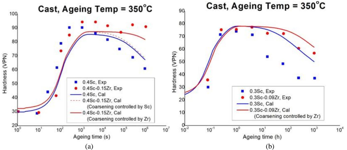
Fig. 7 Comparison of the age hardening curves between (a) binary Al-0.4Sc (wt%) and ternary Al-0.4Sc-0.15Zr (wt%) alloys [21]; (b) binary Al-0.3Sc (wt%) and ternary Al-0.3Sc-0.09Zr (wt%) alloys [22] at cast T5 condition with the ageing temperature of 350°C.
