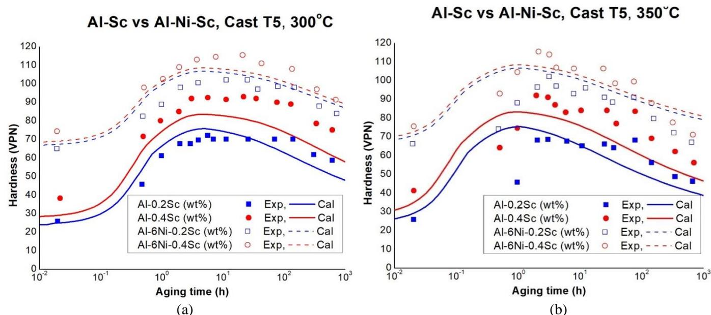
Fig. 6 Age hardening curves of binary Al-0.2Sc (wt%), Al-0.4Sc (wt%) and ternary Al-6Ni-0.2Sc (wt%), Al-6Ni-0.4Sc (wt%) alloys at cast T5 condition [20], with the ageing temperature of 300°C and 350°C.
